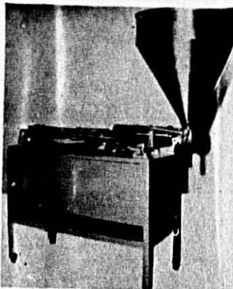
A NEW AUTOMATIC FOOD FILLER with a micrometer adjustment that can increase or decrease quantity of fill while machine operates is announced by the F. L. Burt Co. of San Francisco. The filler can be stopped instantly even in the middle of a discharge stroke without turning off motor switch. Fill liquids or semi-solids at 10 to 30 containers per minute. Adjustable from gallon to 8 ounces. Easily dismantled to clean. Stainless contact or acid resistant nickel alloy contact. 8 foot conveyor optional.
